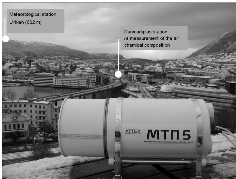
Fig. 1. Meteorological temperature profiler produced by NPO ATTEX (Russia, www.attex.net ). The instrument is installed on the measurement site of the Geophysical Institute of University of Bergen at the height of 45 m above the sea level. The image is dated from February 8, 2011.
