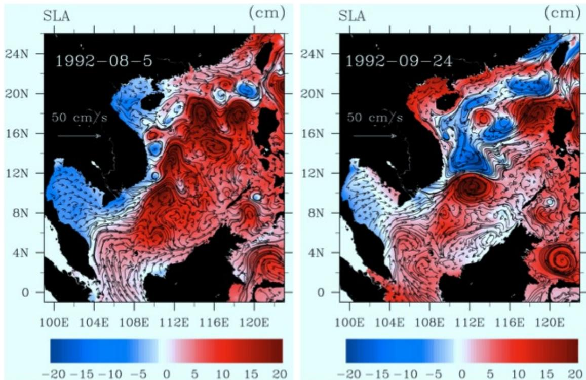
Figure 2: Surface currents and sea surface heights on two typical days in 1992 simulated with the HYCOM 5 km model, showing clear mesoscale dynamic features. Courtesy of Dr. Jiping Xie, IAP, Chinese Academy of Science, Beijing while visiting the MSC.
