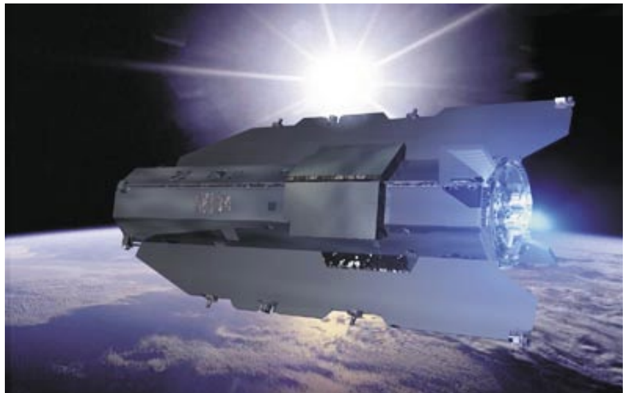
Figure 1b. GOCE octagonal shaped satellite approximately 5 m long and 1 m in diameter (courtesy ESA).
