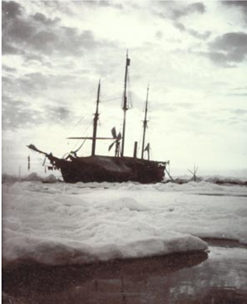
Wind energy gave light to Nansen and colleagues during the Fram voyage in the Arctic Sea (1893-96).
