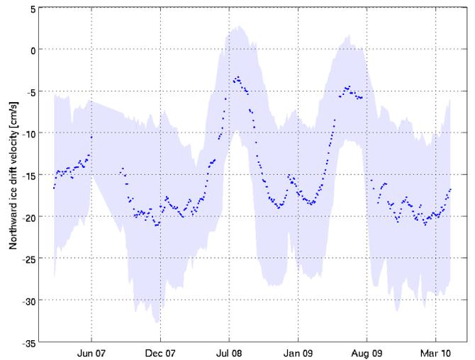
Figure 5. Ice drift velocity component (positive northward) in the Fram Strait across 79° North between 15° West and 5° East, based on feature tracking in ASAR backscatter at 3 days interval and averaged within a 90 days moving window. The purple region indicates one standard deviation within the averaging window.
