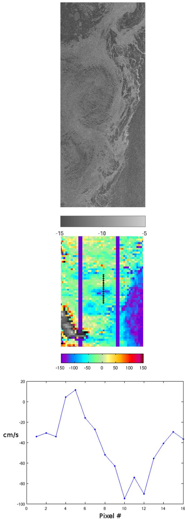
Figure 4. Sea ice eddy observed from ASAR backscatter in the Fram Strait on the 5<sup>th</sup> of November 2008 at 12:01:02 UTC (top), corresponding range oriented velocity measured by Doppler shift (centre), and a profile of the velocity variation (bottom) across the stippled line marked in the centre panel. The distance between pixel centres is 3.2 km, and the Doppler shift only provides relative velocities because of missing land cover in the imaged scene.
