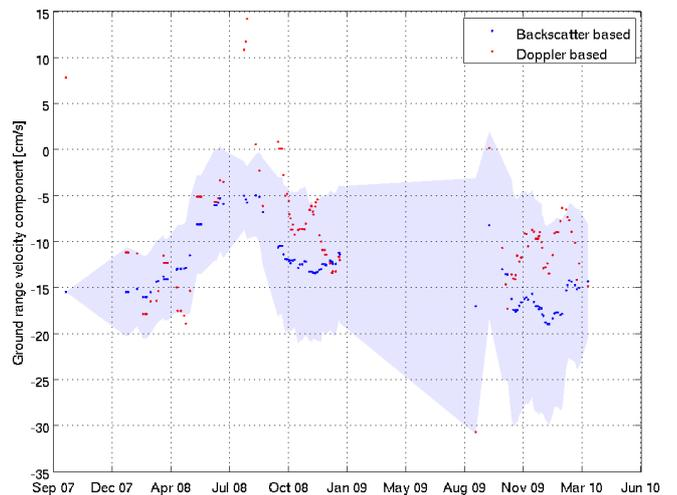
Figure 6. Ground range velocity components across 79° North between 15° West and 5° East based on feature tracking in ASAR backscatter (blue), and ASAR Doppler shift (red). The dataset is smoothed with a 90 days averaging window, and the purple region indicates one standard deviation of the radar backscatter based data within this averaging window.
