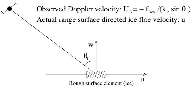
Figure 1. Interaction between a rough surface element (in this case ice), and the radar signal at incidence angle  $\theta_I$  with ice floe velocities  $u$  and  $w$  in ground range and vertical direction, respectively. The Doppler velocity ( $U_D$ ) is a function of the Doppler anomaly ( $f_{Dca}$ ), the electromagnetic wave number ( $k_e$ ), and the incidence angle ( $\theta_I$ ).
