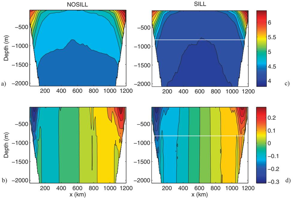
Figure 3. Zonal sections at the mid-latitude of the marginal sea: temperature (in °C; upper panels), and meridional velocity (in  $\text{m s}^{-1}$ ; lower panels) for NOSILL (a, b) and SILL (c, d). Contour interval is  $0.2\text{ }^{\circ}\text{C}$  for the temperature, and  $0.05\text{ m s}^{-1}$  for the velocity. White lines indicate sill depth.
