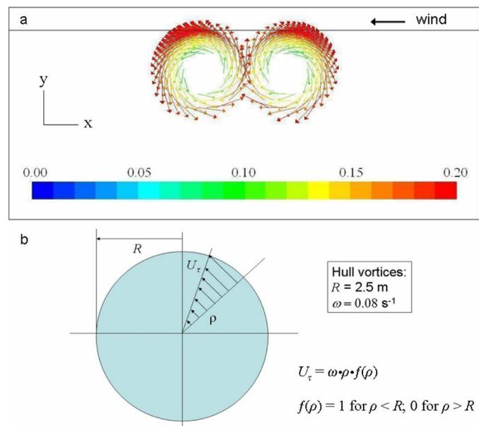
Fig. 1. (a) Initial velocity vectors of counterrotating vortex pair colored by velocity magnitude (meters per second); (b) radial structure of the vortex.
