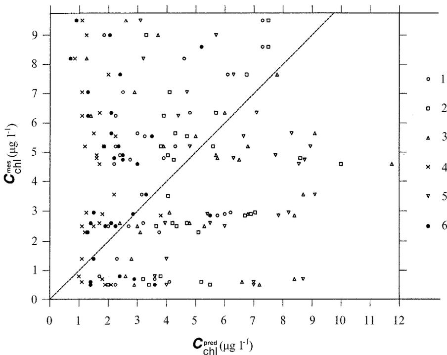
Figure 11. Directly-sampled chl concentrations in Lake Ladoga plotted against chl concentrations predicted by six different oceanic chl-retrieval algorithms taken from Gordon and Morel (1983).
