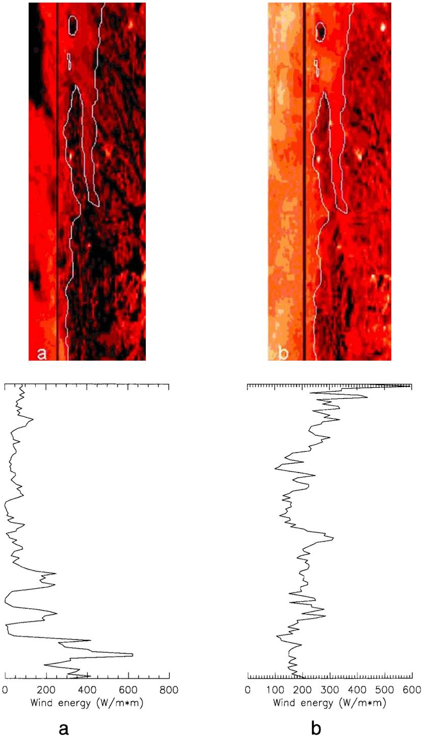
Figure 3. Wind energy maps (top) from two different ERS-1 passes and the corresponding variations in energy variation along a profile at 10 m height following the black vertical line in the two top figures. The selected area is indicated with a yellow rectangle in figure 2 (b).
