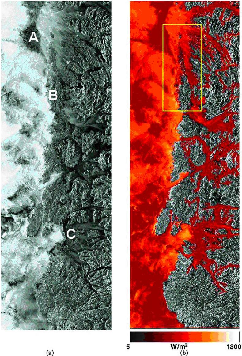
Figure 2. SAR image from Norwegian west-coast (left) and corresponding map of wind energy at 10 m height (right). Brighter areas indicate more wind energy.
