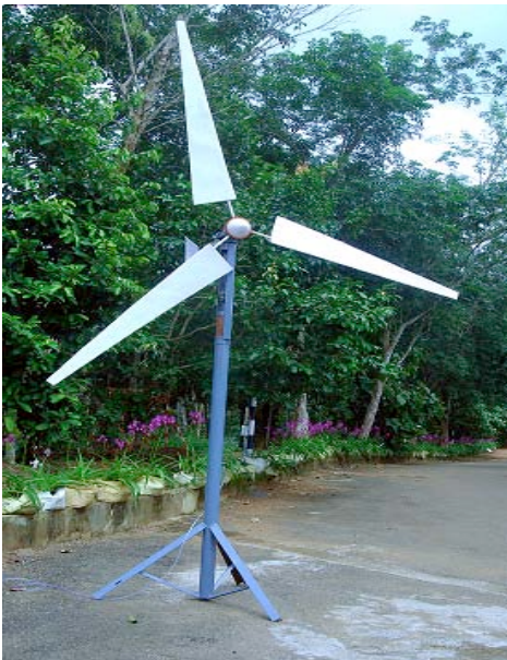
Wind induced aerator system for water quality improvement in canals and lakes developed by Dept. of Mechanical Engineering, ToC institute of Science and Technology in collaboration with NERCI under UNEP-APFED project.
